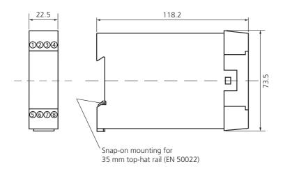
Captive M3x8 clamping screws, box terminals with self-releasing wire protection, max. conductor cross-section  $1 \times 4 \text{ mm}^2$  solid;  $1 \times 2.5 \text{ mm}^2$  stranded with ferrule;  $2 \times 1.5 \text{ mm}^2$  stranded with ferrule
